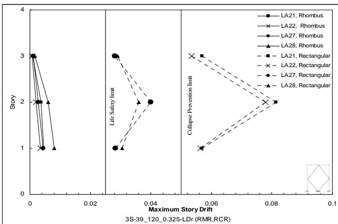
Figure 4. Inter story drift for earthquakes with 2% probability of exceedence in 50 years.
