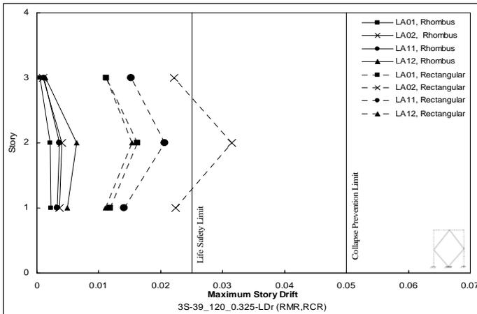
Figure 3. Inter story drift for earthquakes with 10% probability of exceedence in 50 years
